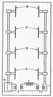
Method of assembling spaced dipole aerials for direction finding.
