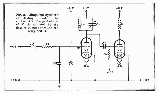
detected in a nearby oscillating receiver), then from the value of this critical bias voltage the value of the RF resistance may be found directly from the curve, oscillations ceasing when the negative resistance becomes equal to the dynamic resistance of the tuned circuit.
