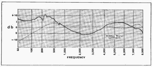
Response curve of Shure Model 99A crystal pick-up with 0.5 M $\Omega$ , shunt. Zero db is equivalent to 1 volt RMS and the dotted curve shows the characteristic of test record.
