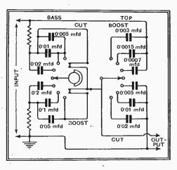
3.—A composite circuit providing control of both bass and treble. Fig.
