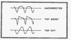
Fig. 8.—Waveform distortion caused by a saturated valve.
