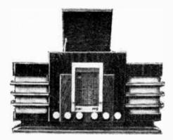
Modern French cabinet design : the speaker of the Lemouzy receiver is mounted horizontally, with an adjustable reflector above it.
