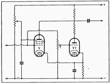
Arrangement of amplifying valves in television apparatus to correct for distortion.
