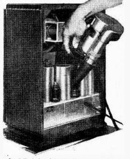
Specially designed for blowing dust out of the nooks and crannies of a receiver chassis, this American machine is fitted with an insulating nozzle of soft rubber that cannot damage delicate parts.
