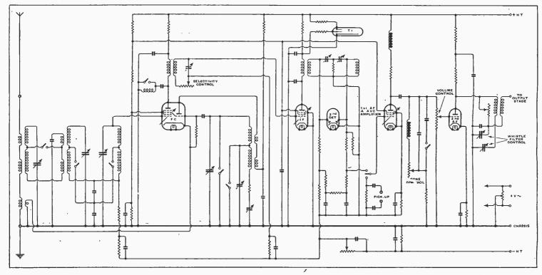
Circuit diagram of receiver chassis. The output stage and power pack have been omitted as their connections are straightforward apart from the fact that the -HT lead is below earth potential.
