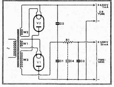
Fig. 37.—With the voltage-doubler rectifier it is possible to run the time-base, as well as the tube, from the HV unit in the manner shown here.
