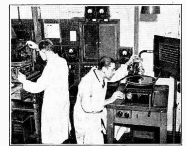
Two of the four machines used by H.M.V. for recording the Coronation ceremony and the King's speech. These were employed in pairs to minimise the chances of a failure, and to insure continuity the second pair came into operation before the first had completed a record.
