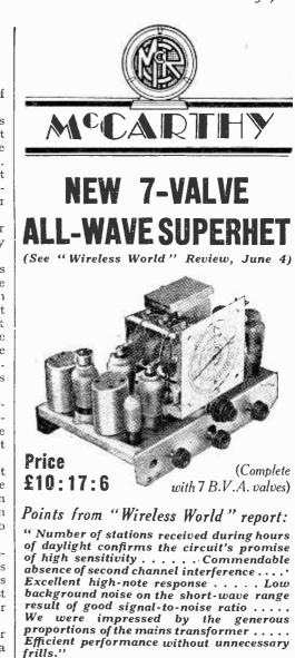
**Circuit details :** Aerial input to high-gain R/F amplifier. Triode-hexode frequency changer coupled by air-cored high efficiency I.F. transformer to I.F. amplifier. Diode detector with delayed A.V.C. L.F. amplifier and 4 watt output pentode. Sockets provided for ext. speaker and gram pick-up. 4-position wave-change and gram switch. Vol. control and variable tone control operate on radio and gram.
