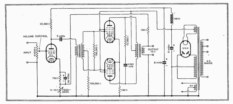
Fig. 3.—Circuit diagram of complete amplifier. With slight modifications a tone control stage giving exceptionally comprehensive adjustment of tone and, if needed, extra gain, can be added. Details will be given later.
