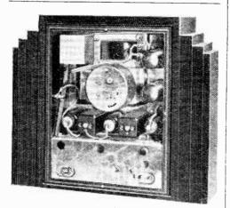
Back view of Radiochron showing all-metal valves grouped round central synchronous clock movement. The hands are driven through the hollow pole-piece of the moving-coil loud speaker.
