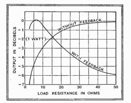
Fig. 6.—The effect of negative feed-back on the output/load resistance characteristic of the amplifier described. These curves do not take account of distortion, which is excluded by running well within the rated output.
