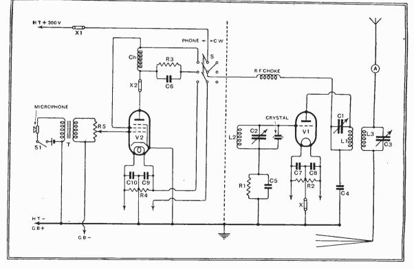
Fig. 1.—Circuit diagram for the transmitter, showing change-over switching for morse or 'phone. With centretap keying as shown (key at X), separate LT windings are necessary for V1 and V2. With certain valves, conditions may arise where it is better to connect the screen of V2 to the anode side of the choke.
