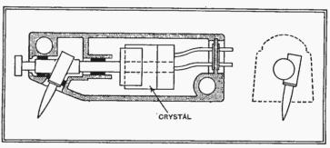
Diagrammatic section and end view of Shure pick-up showing tilt of needle in two planes.
