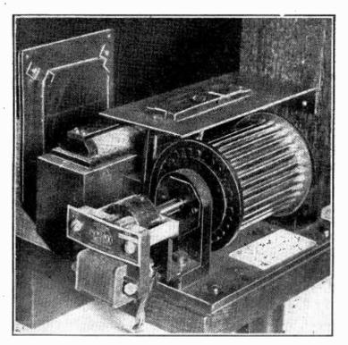
man's head with banks of photo-cells on either side, and in front of it a spot-light mirror-drum scanner. On the other side of the booth is the mirror-drum receiver. Baird have also on view a large cathoderay tube designed for electromagnetic defive mounted in the form of an arc, and the rotating element is a nine-sided poly-
