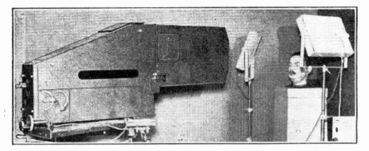
The Baird 30-line Spot-light scanner which was used in the B.B.C. transmissions up to 1932. The banks of photo-cells can be seen on either side of the head.
