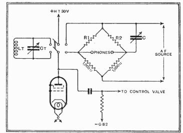
is varied until a minimum is heard in the phones, and the C is adjusted to give a better minimum. R2 is then set for final balance. The negative resistance  $R^{i} = \frac{R_{I} R_{2}}{R_{I} + R_{2}}$
