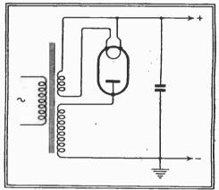
Fig. 34.—The same half-wave rectifier with negative HT earthed. This increases the voltage between the transformer windings.
