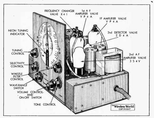
Controls are clearly marked and mounted on the large ivorine tuning panel.
