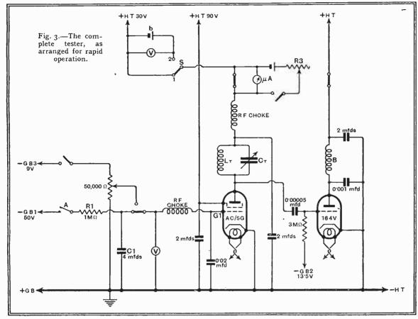
it allows the condenser CI to charge up through the resistance R1, applying a gradually increasing voltage to the control grid GI of the dynatron, the value at any instant being recorded by the voltmeter V.
