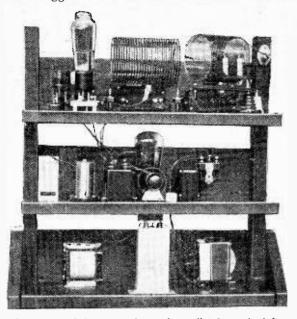
Rear view of the transmitter : immediately to the left of the oscillator valve on the top shelf is the combined grid coil and crystal holder; a valve base is used for this purpose.
