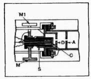
Constructional details of C.R. tube with adjustable cathode.
