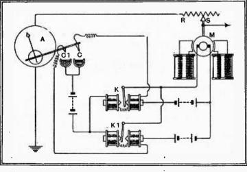
Fig. 1.—Automatic control of signal current as applied to landline communication.
