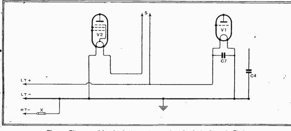
Fig. 2.—Filament wiring for battery valves; other circuit details as in Fig. 1.
