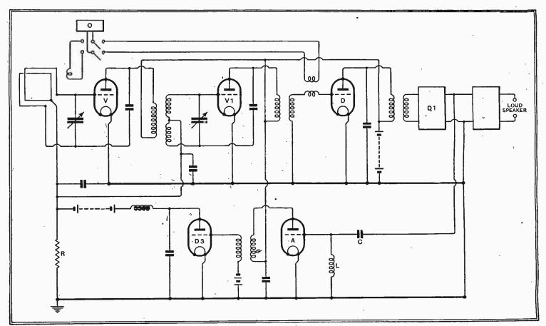
Fig. 2.—An early method of controlling the gain of an RF amplifier
